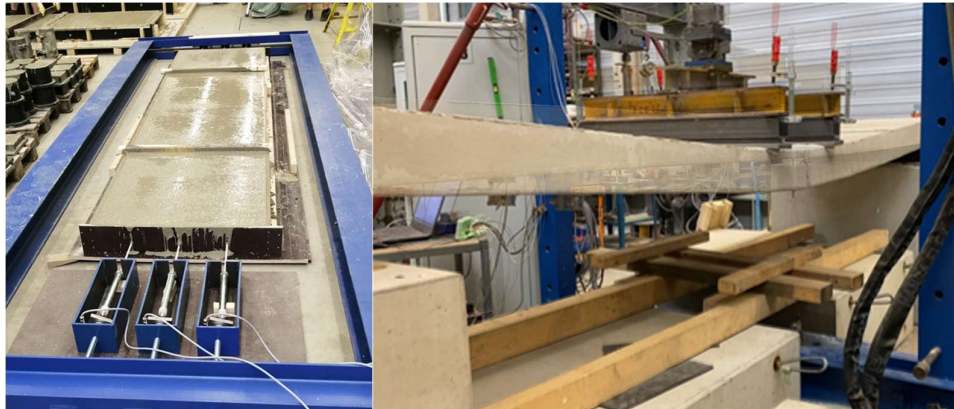
Figure 2-6: Manufacturing and testing of a member with prestressed GFRP tendons
